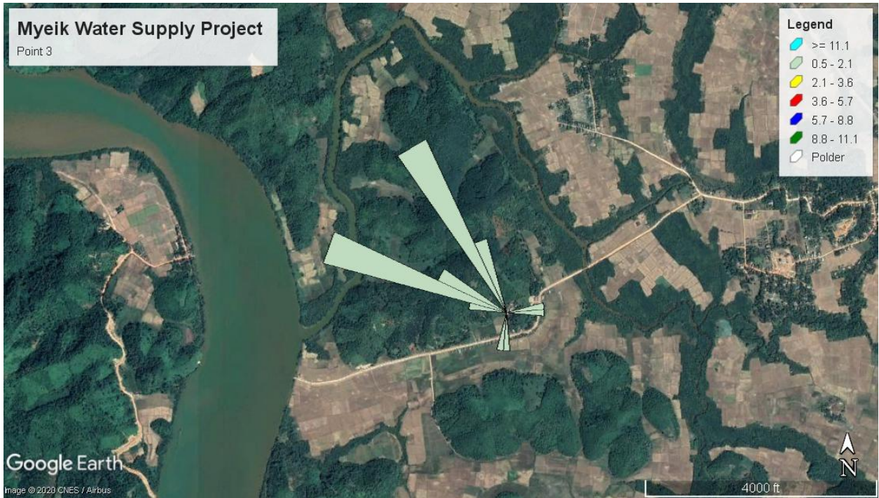
Figure 5-46 Wind Speed and Wind Direction (Blowing from) at Point 3 (Tone Byaw Gyi Village for Wet Season)
