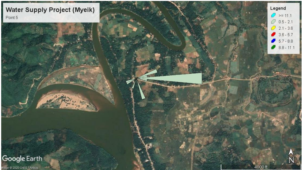
Figure 5-52 Wind Speed and Wind Direction (Blowing from) at Point 5 (East Maw Tone Village for Dry Season)
