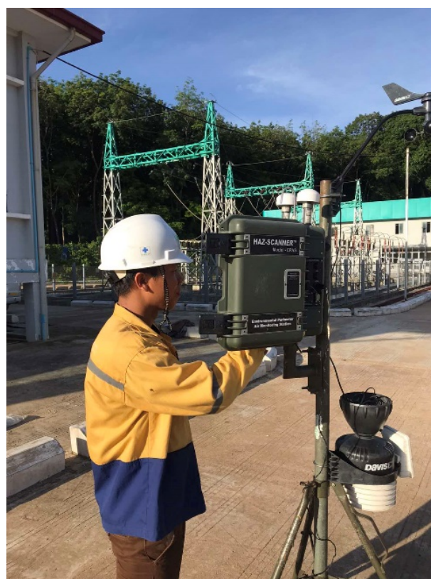
Figure 6- 7 Air Quality Measurement near transmitters at the project site
