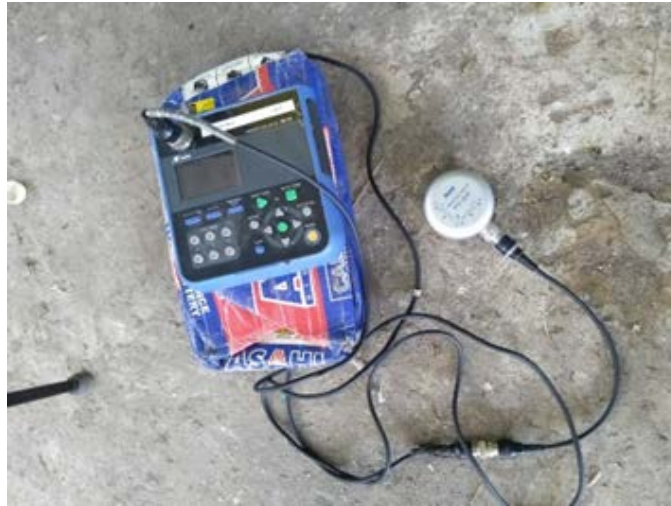
Figure 6- 15 Vibration Survey Point at project site
