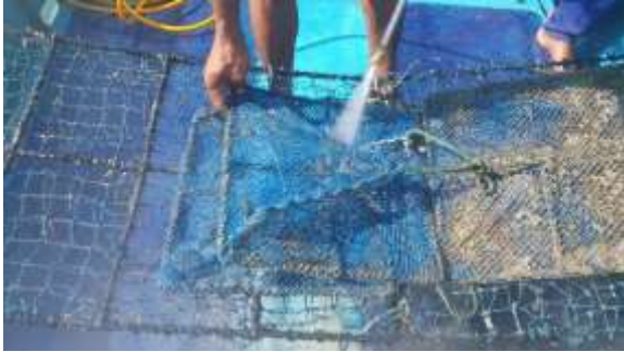
Figure 5-10 Cleaning triangle nets using high pressure cleaner
